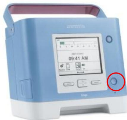
To stop ventilation again press the power button on the front of the ventilator. When turning off, you will be asked to confirm you wish to power down the ventilator.
